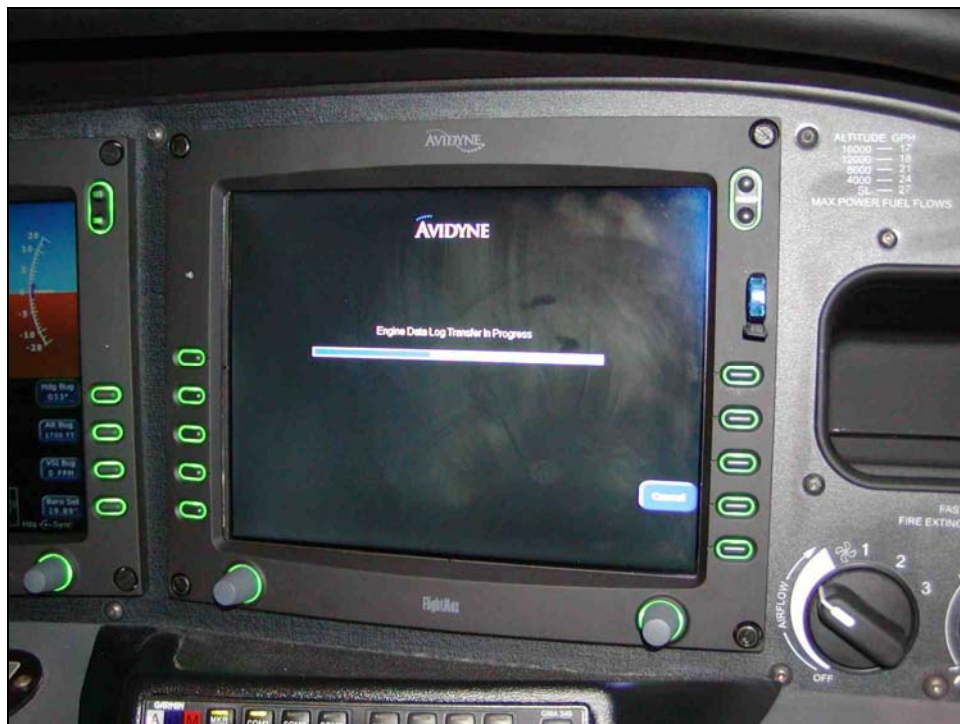
Figure 4. FlightMax display showing data transfer progress status.
