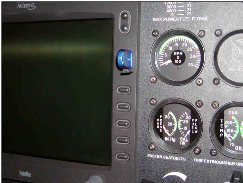
Figure 2. USB Thumb Drive Inserted in Avidyne FlightMax.
