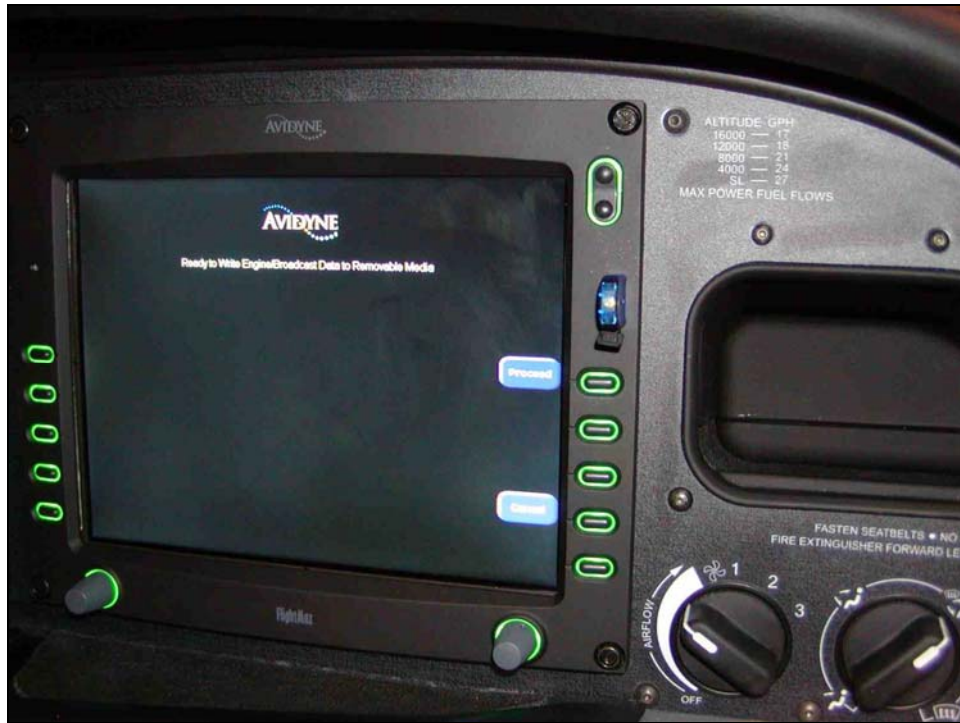
Figure 3. FlightMax display after starting with ThumbDrive inserted.
